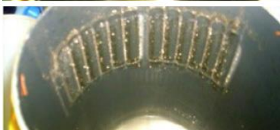
Nibral particles captured by FilterMag in each of the four high pressure filters.
