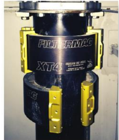
Four FilterMag XT4s we installed on the cartridge filter of a trunnion gear oil system supporting a large ball mill.
