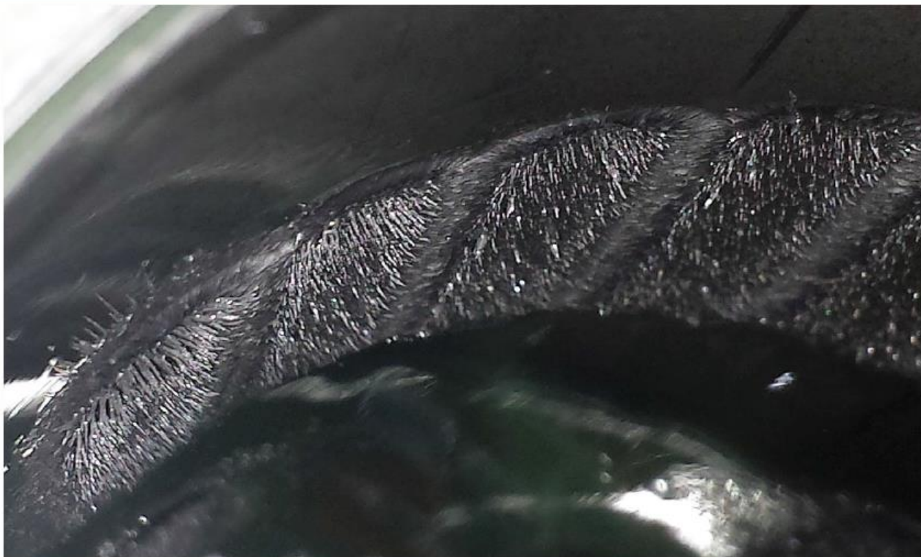
Stage 1 Closeup—The Nature of Partical Stacking in a Magnetic Field
