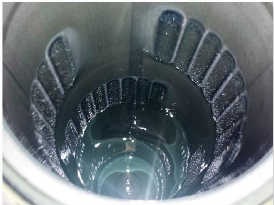
Stage 2: Normal wear will show a light dusting of captured particles.
