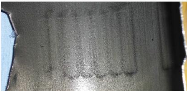
Photo of particles caught by FilterMag on inside of filter canister.
